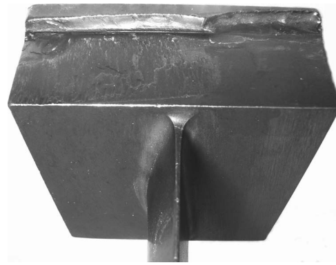
Fig. 2 Stator vane damage
